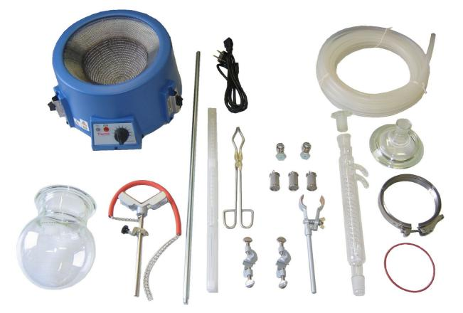
2. Place the flask into the heating mantle and fasten by means of the provided chain clamp.
