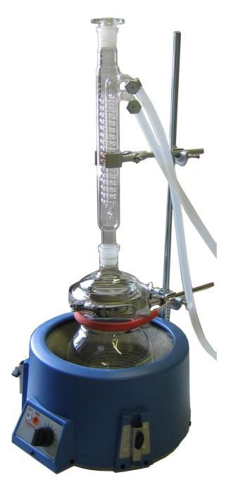
8. Connect inlet and outlet hose of the Dimroth cooler with water supply and drain. Cooling power is to be adjusted directly from the domestic water faucet.
