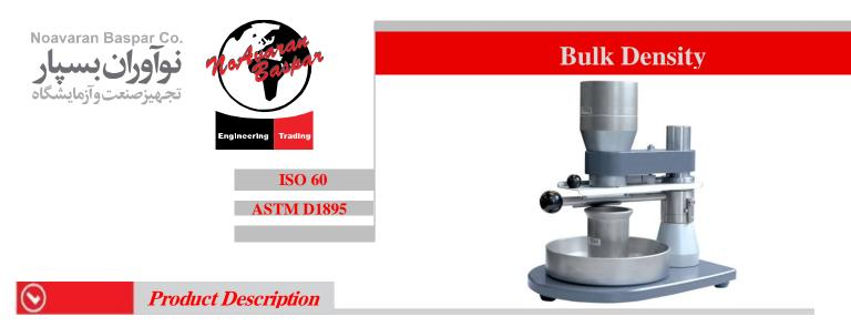
This instrument has been built using high quality materials and consists of a filling funnel with a spring-loaded trap, a plate with tripod and a graduated measure jug with a drip cup. The massive weight of the body provides good stability for the funnel, which can contain approximately 200 ml.
